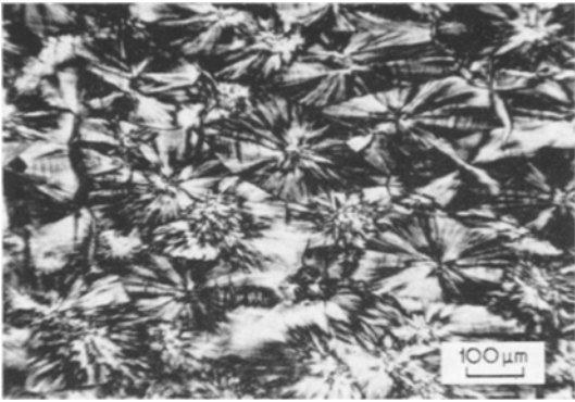
Figure 5 Striations in necked region in the form of arcs perpendicular to and oriented along the stress direction. Stress direction horizontal at 60% overall strain and 70% maximum strain in necked region.
